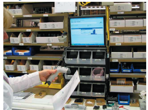
Scanning traceability information from job ticket before final calibration checks are done.
